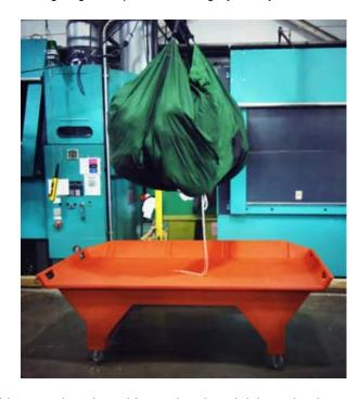
This rugged sorting table can be placed right under the overhead rail system for handling the sling discharge, sorting and conveying. It can catch up to 400 lbs. of goods and is rotationally molded in one smooth piece of 100 percent
