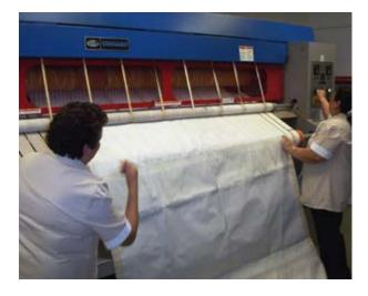
Put away the sandpaper and tell your workers to stop scraping and scrubbing the cylinders. The new Kleeno Cylinder cleaning pad is the first and only cleaning pad material designed specifically for cleaning cylinder ironers. Just feed it into the ironer and it automatically removes dirt, grime and chemical buildup in a few short minutes. Potentially dangerous, manual cleaning is no longer required.
